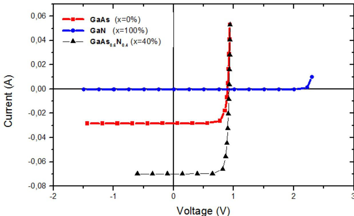
**Figure 2** Current-voltage characteristics of the three p-n junction solar cells based on GaAs<sub>1-x</sub>N<sub>x</sub> for  $x = 0\%$ ,  $x = 40\%$  and  $x = 100\%$ .
