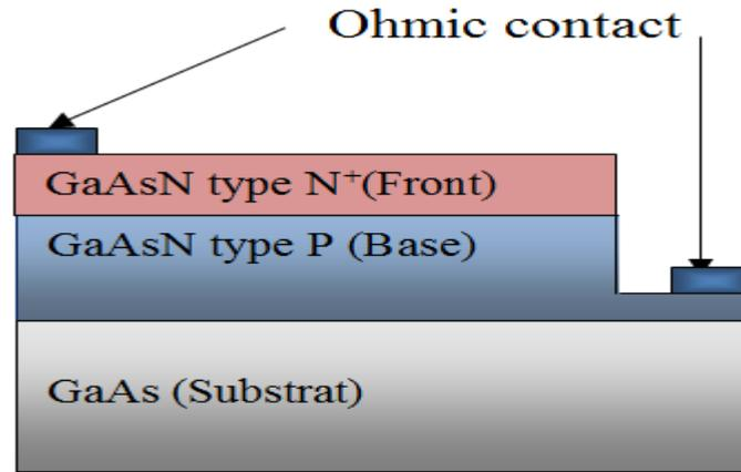
**Figure 1** Presentation of the GaAsN based p-n junction solar cell.
