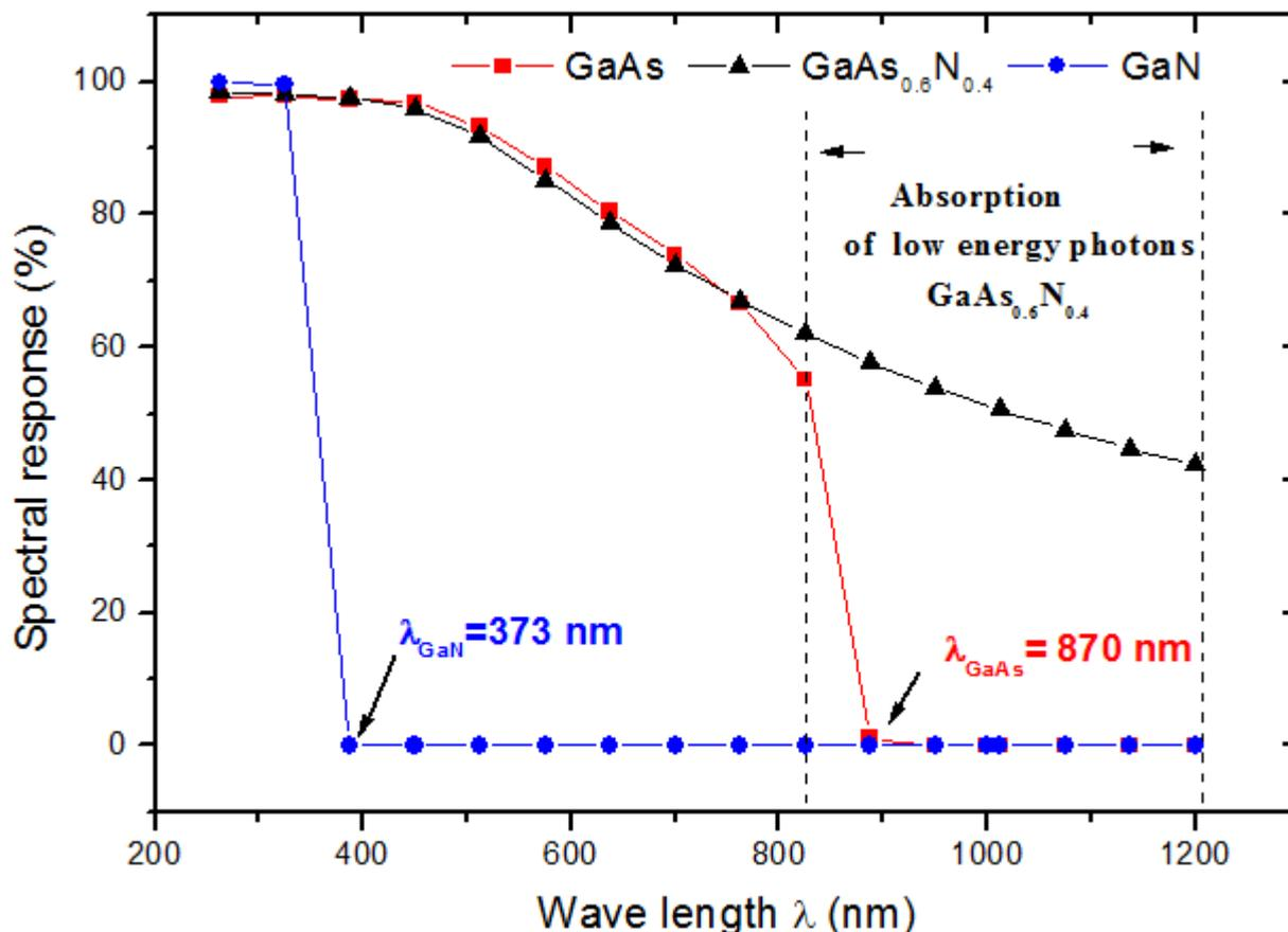
**Figure 3** The spectral responses of the three p-n junction solar cell GaAs, GaAs<sub>0.6</sub>N<sub>0.4</sub> and GaN.
